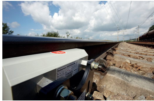
Frauscher Wheel Sensor RSR180 mounted with rail claw
